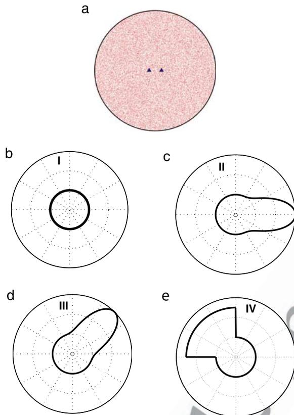
**Figure 13.** (a) Circular region with a diameter of 4000 km for the noise simulation. Each red dot represents a randomly distributed source. The two blue triangles are the two receiver stations placed 450 km apart. (b–e) Azimuthal distributions of the strength of source energy delineated by the bold lines for experiments I, II, III, and IV, respectively.
