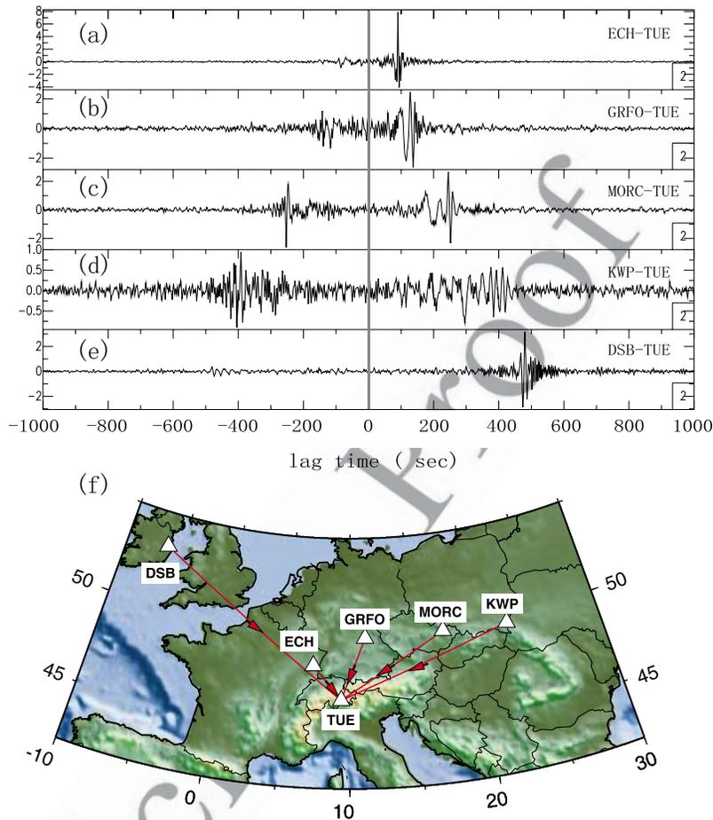
**Figure 2.** (a–e) Examples of 12-month broadband cross correlations. The bold gray line indicates the zero arrival time. Cross correlations are ordered by interstation distances with station names indicated in each waveform panel. Note that the cross correlations are often asymmetric. (f) Locations of the stations (white triangles) and path segments for the corresponding cross correlations, with arrows marking the incoming directions of noise contributing to the positive components.
