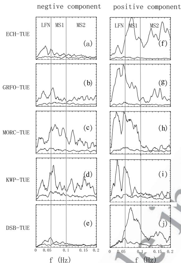
**Figure 3.** Normalized spectra of (a–e) negative and (f–j) positive components of the cross correlations shown in Figure 2. The three frequency bands of LFN, MS1 and MS2 delineated by the bold lines correspond to the infragravity band and the primary and secondary microseism bands.
