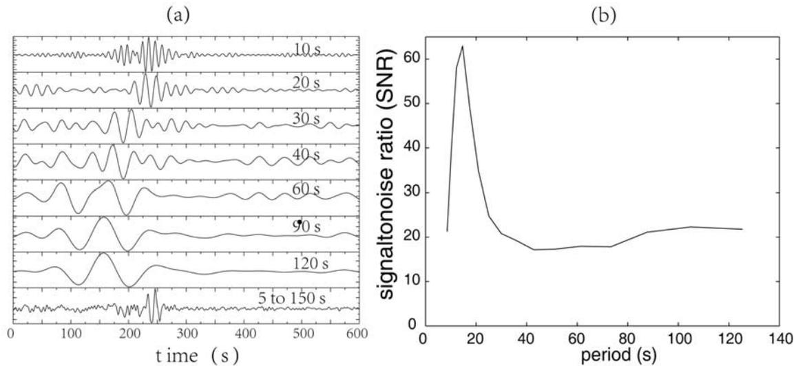
**Figure 4.** (a) Example of a broadband positive component cross correlation using 12 months of data between stations IBBN (Ibbenbueren, Germany) and MOA (Molln, Austria). The broadband signal (5–150 s) is shown in the eighth panel. Other panels are narrow band-pass filtered waveforms with the central periods indicated in each panel. (b) Calculated SNR values from each narrow band-passed filtered waveforms versus period.
