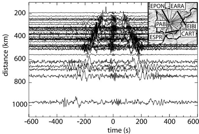
**Figure 2.** Record section of raw (unfiltered) cross correlations of stations in the Iberian Peninsula with respect to station PAB obtained using 4 months of ambient noise data. The causal (positive time) and acausal (negative time) arrivals of the Rayleigh wave are clearly visible in all records. The inset shows the location of the paths corresponding to the record section shown in this figure (thin gray lines) and of the group velocity measurements shown in Figure 3 (thick black lines).
