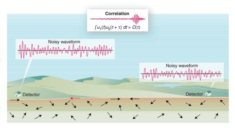
**Using noise in seismology.** When a diffuse wave field is generated by distant sources and/or by multiple scattering, detectors report random signals. Occasionally a ray (for example, the one shown in red) passes through both detectors. As a result, the signals are weakly correlated.
