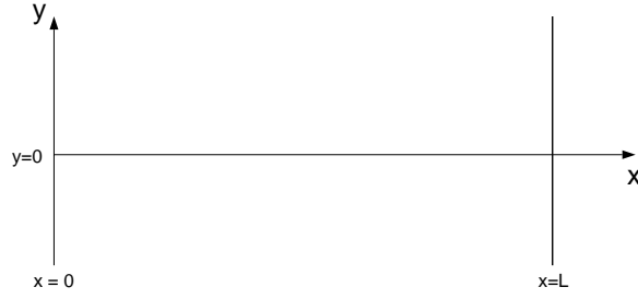
Figure 5: Coordinate system for a string of length L that will undergo vertical (or transverse) displacements y(x, t) .
